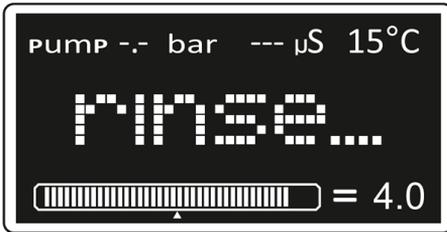
6. Then pause the rinsing process and connect the outlet water hose to the system to be filled.
