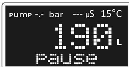
4. Press the circle button to start the rinsing process. The rinsing process takes approx. 60 seconds. Following the rinsing process, the production of outlet water begins and the LED indicator remains lit up in green.
